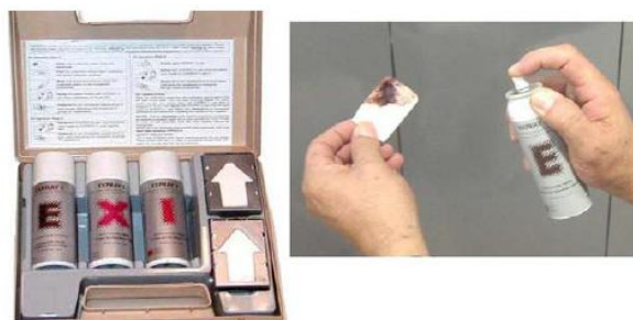
Figure 5. Expray reagent kit and application [11]
