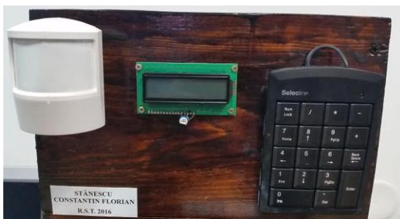
Figure 6. Implemented system frontal view with keypad, LCD and motion sensor.
