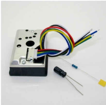
Figure 7. Air Quality Module
